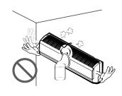
When flammable gas leaks, turn off the gas and open a window for ventilation before turn the product on.
